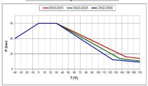
The given data of the pressure-temperature chart refer to the valve body
